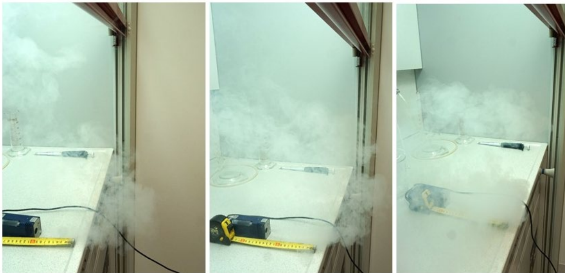
Figure: Smoke tests during work in the fume hood ZK1 1.323 biochemistry in which smoke was blown into the sash opening of the fume hood was blown in at 3 different distances from the sash opening (left photo 10 cm, middle photo 15 cm and right photo 20 cm).
