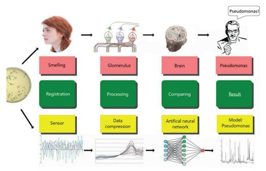
Figure 4. Comparison of the steps required to detect an odor using either a biological nose or an e-nose. Reprinted and adjusted from **Transferable Odor Differentiation Models for Infectious Disease Diagnostics**, 2014, M. Bruins, The Electronic nose, Page 16, with permission from M. Bruins ISBN 978-94-6108-600-6
