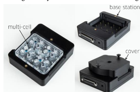
Figure 1: The multi-cell is mounted in a base station and fixed by the cover, which is used to press the rear-side contact of the sensors onto the spring-loaded contact pins.
