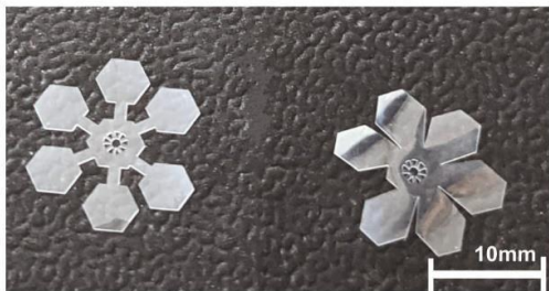
Figure 1: The new concept for foldable and flexible epiretinal implants with multiple functionality. First test structures were realized in Parylene-C.
